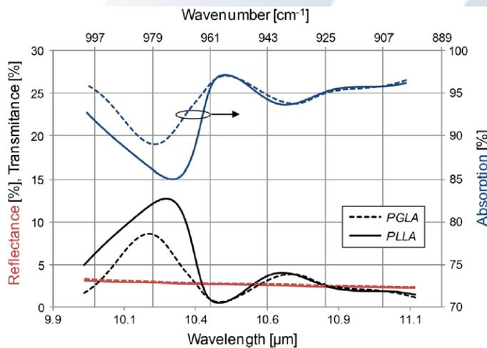
Figure 2: Transmittance, reflectance and absorption spectra of 250µm thick poly(L-lactide and poly(L-lactide-co-glycolide) sheets.
