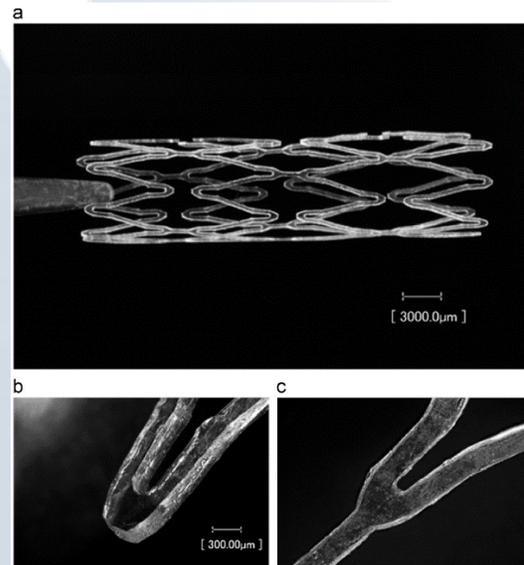
Figure 3: An example of a vascular stent made by CO<sub>2</sub> laser micromachining: (a) the entire stent with a metric scale, (b) and (c) magnification of selected areas of stent struts.
