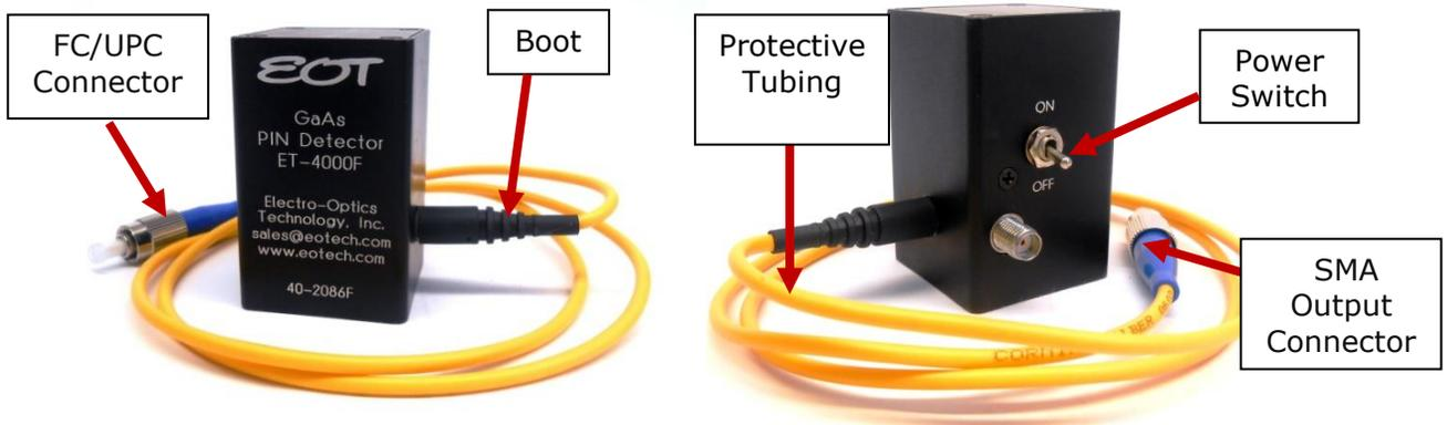
When terminated into 50  $\Omega$  into an oscilloscope, the pulsewidth of a laser can be measured. When terminated into a spectrum analyzer, the frequency response of a laser can be measured.
