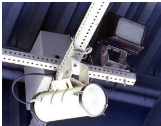
Figure 4: Proof of concept hardware includes camera, lighting and control modules. Hardware is mounted on the underside of an overpass or bridge and is triggered by a laser vehicle location system (not shown)
