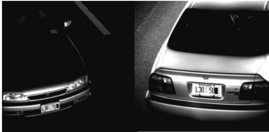
Figure 2: Typical images acquired from high speed toll system on the New York State Thruway system. Both front and rear license plate images are acquired at full highway speed with sufficient resolution for the OCR engine to read the numerals. The plates may be located anywhere within the field of view. (The last numeral has been intentionally blacked out)
