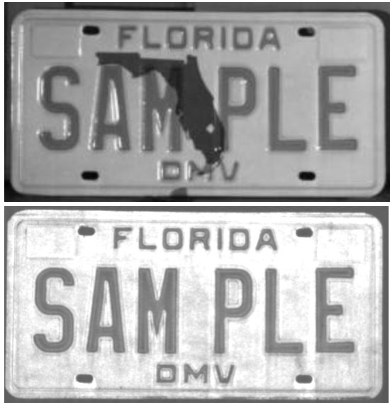
Figure 7: Variation in images of sample plate showing the effects of different lighting schemes. The top plate is illuminated under white light, the bottom one using NIR illumination. For properly designed plates the contrast is greatly improved for automated OCR reading using NIR illumination. Note that proper design makes possible the use of visible graphics that make recognition difficult under white light schemes.
