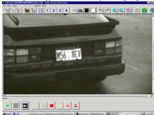
Figure 5: The Toll Enforcer™ software combines OCR processing with manual verification reports that link reports directly to DMV database protocols.
