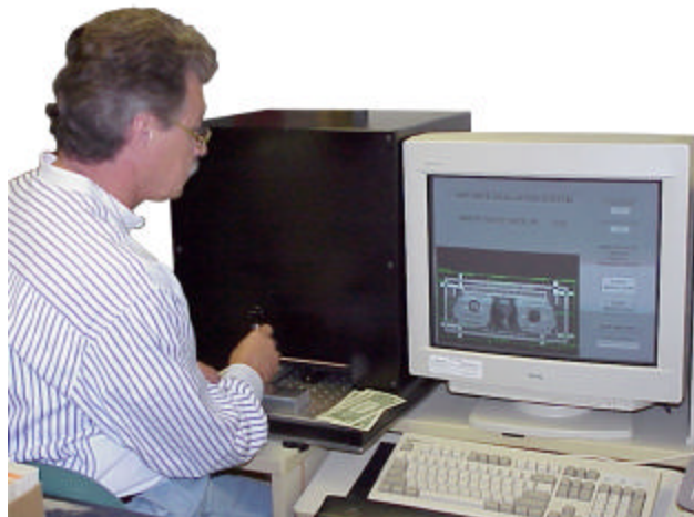
Figure 6: Note Measurement System provides highly accurate data on currency stability and registration and is instrumental in understanding the intricacies of the manufacturing process
