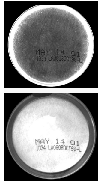
Figure 12: Concave SBI provides high contrast brightfield illumination for objects that have concave domed or depressed regions.
